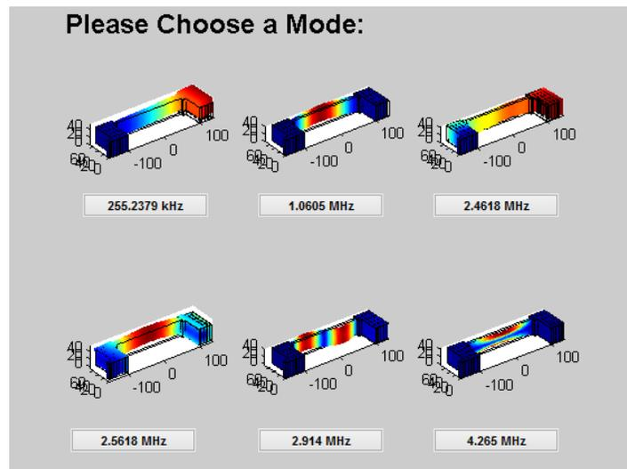
Another method of recognizing the mode shape is to pick a surface (or surfaces) that experiences a large normal displacement. Two options are available for this: in-plane and out-of-plane. The code then selects the mode with the maximum squared relative displacement on that surface. For this, the *Autotrack Surfaces* field must be filled, and the *Mode Type* field must be specified as *In Plane* or *Out of Plane*. The desired mode should be within  $\pm 20\%$  of the specified frequency.
