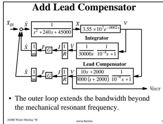
Thus far, we have measured the sensitivity and resolution of our capacitive geophone with integral feedback. The story could be done, expect that now the frequency range is limited at the high end by the resonance of the mechanical system. Since conventional geophones are typically used at frequencies well above their resonance, we have added a lead controller to extend the bandwidth.
