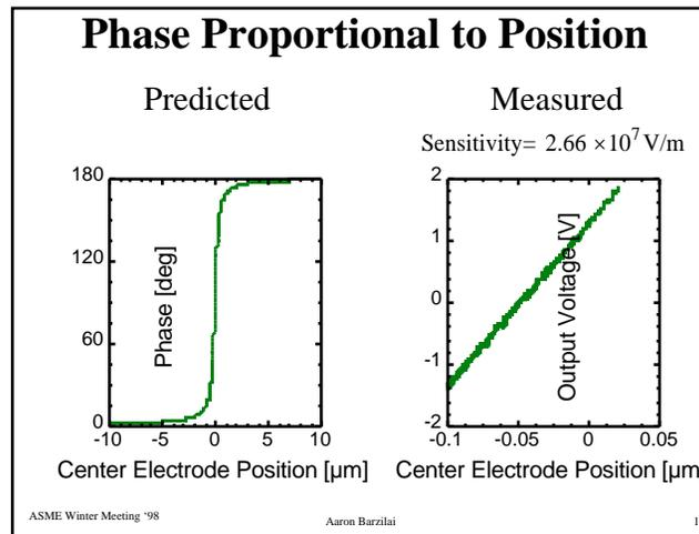
It turns out the phase is the signal we're most interested in. You can see the relationship is non-linear, with the highest sensitivity occurring when the gaps are balanced. Our experiments have shown that in practice we obtain very high sensitivity of about 25 MV/m or 25 V/ $\mu\text{m}$ , and that in the center the relationship is approximately linear.
