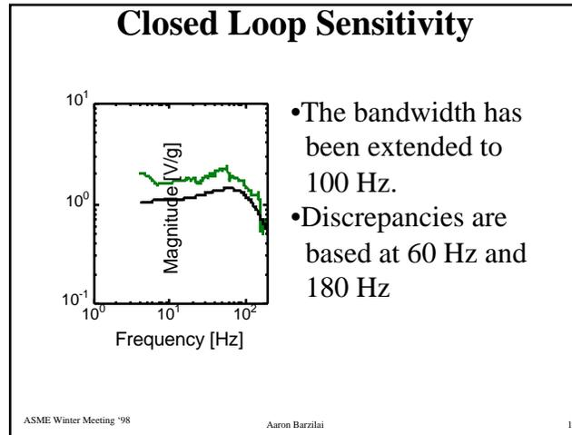
For our present controller, the model predicts a high frequency rolloff at 100 Hz. Our data seems to match this prediction, but there are some discrepancies. First, we have a constant error in our predicted sensitivity. Secondly, at 60 Hz and 180 Hz there are discrete jumps in the sensitivity. We believe this result is promising, but measurement errors are causing the discrepancies. We will continue to study this until our experimental results match our prediction.
