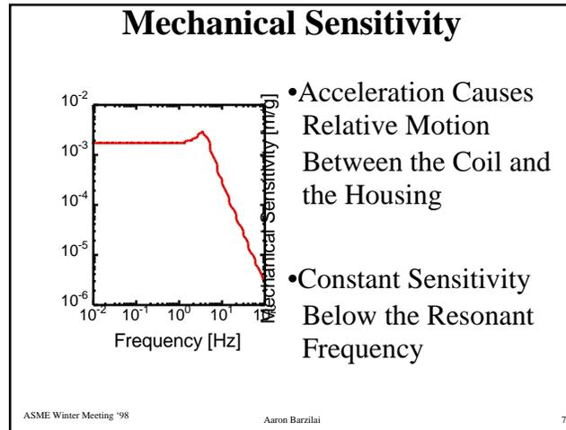
The mechanical system, which converts the input acceleration into relative motion, behaves like a typical second order system. Below the resonant frequency, the sensitivity is constant. Above the resonance, the sensitivity falls off at 40 dB/decade.
