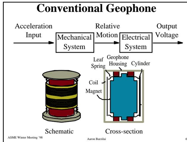
So, let's take a look at how a geophone works and why it is currently used in high frequency applications. I have a sketch of the inside of a geophone and a cross-section. Remember, a geophone is cylindrically symmetrical.
