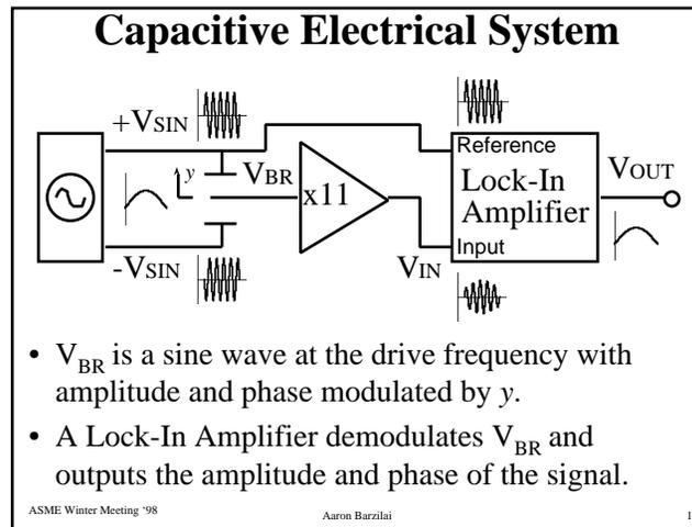
To measure the motion, we apply sine waves approximately 180 degrees out of phase from each other to the fixed electrodes. The motion of the proof mass causes a modulated version of the driving sine wave to appear on the center electrode. This signal and the driving sine wave is fed into a Lock-In amplifier, which outputs the amplitude and phase of the signal at the center electrode.
