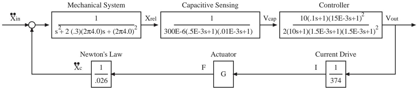
Figure 8: Block diagram of closed loop capacitive geophone system
