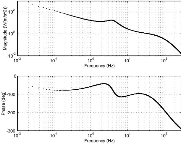
Figure 11: Predicted loop gain of closed loop geophone controller
