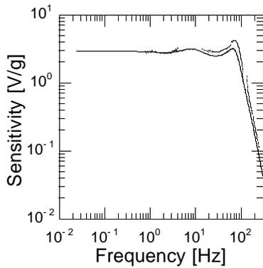
Figure 12: Predicted(-) and measured(.) sensitivity of a closed loop capacitive geophone
