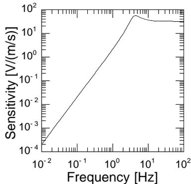
Figure 3: Predicted sensitivity of an OYO Geospace 4.5 Hz GS-11D geophone to velocity
