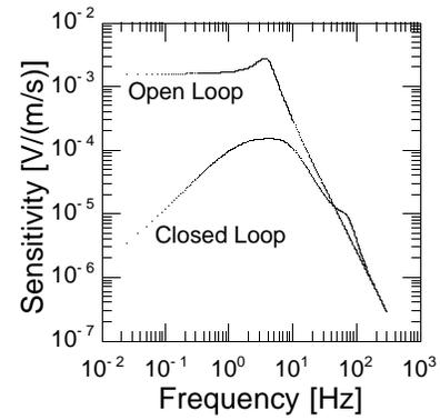
Figure 13: Predicted transfer function between geophone proof mass and input acceleration when operated as an open loop and closed loop sensor
