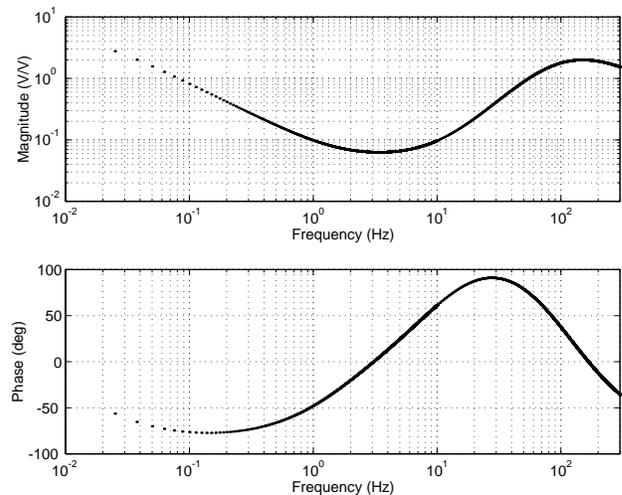
Figure 10: Predicted open loop frequency response of closed loop geophone controller
