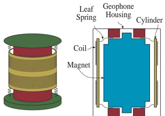
Figure 1: Schematic drawing and cross-sectional view of a geophone
