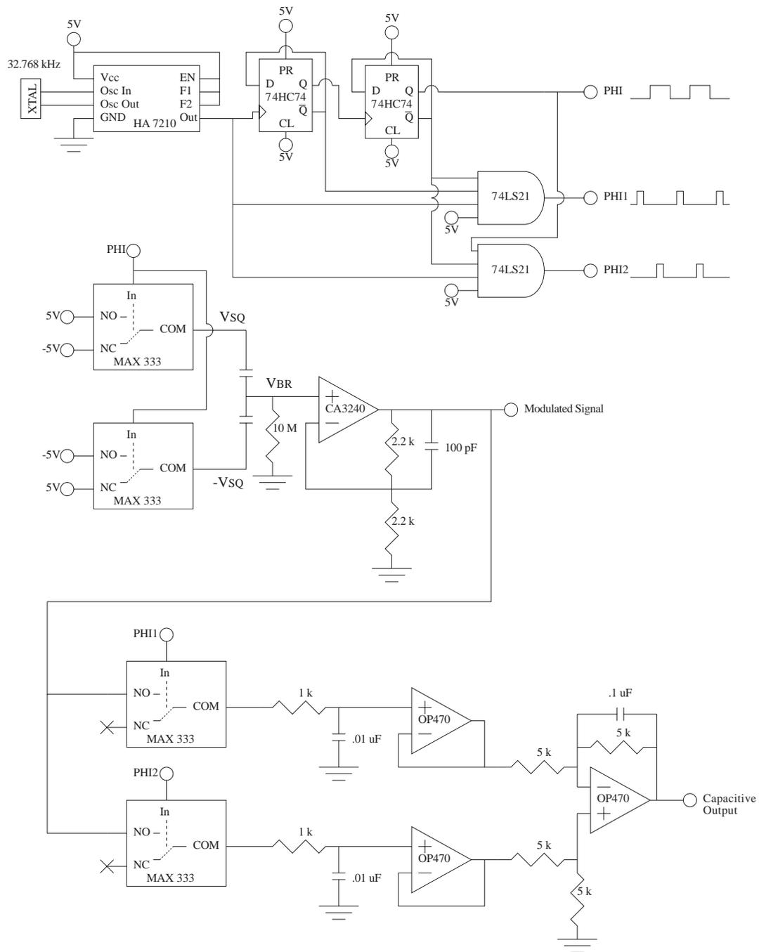
Figure 5: Circuit for capacitive position detection
