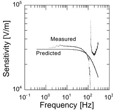
Figure 6: Predicted and measured sensitivity of capacitive position detection
