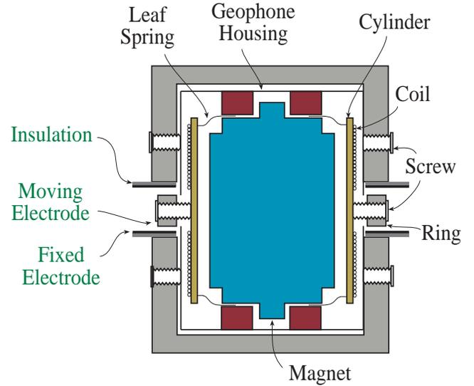
Figure 4: Cross-sectional view of a capacitive geophone(not to scale)
