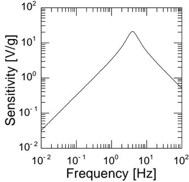
Figure 2: Predicted sensitivity of an OYO Geospace 4.5 Hz GS-11D geophone to acceleration
