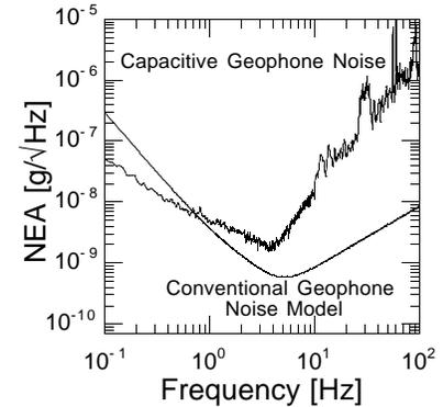
Figure 7: Measured noise equivalent acceleration(NEA) of a capacitive GS-11D geophone and predicted NEA of a conventional GS-11D
