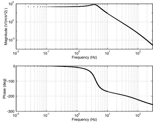
Figure 9: Predicted capacitive geophone open loop frequency response
