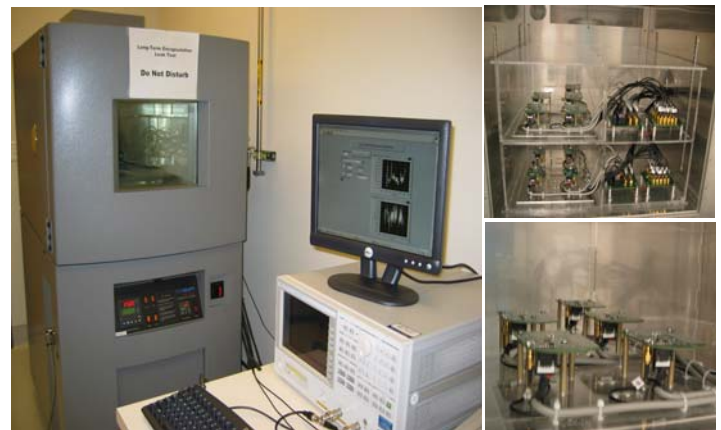
Figure 5 Test setup for long-term stability test. Resonators are installed in parallel in the temperature chamber which maintains the temperature constant environment.
