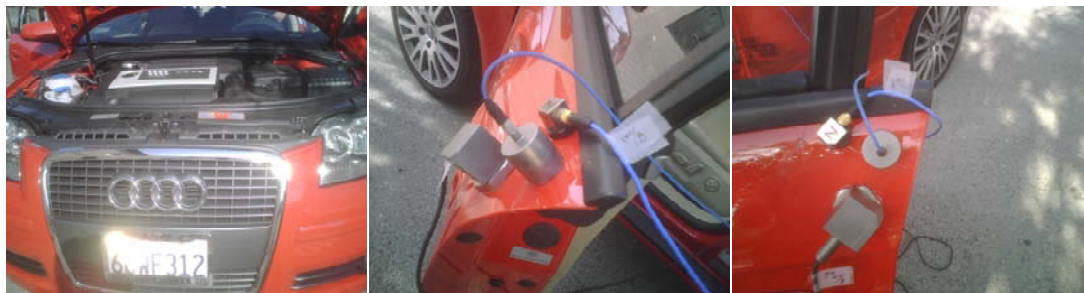
Fig. 7.1: Vibration measurement of a running (engine turned on) car by attaching accelerometers at various locations.
