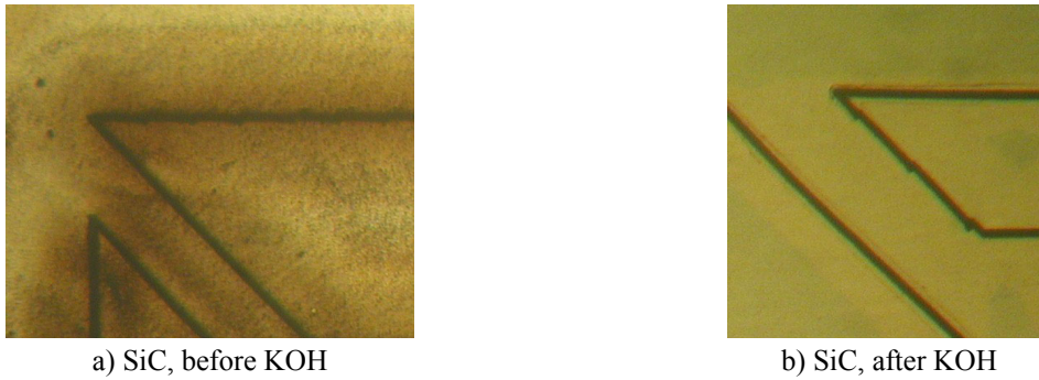
Figure 36 Laser debris, before and after KOH etching.
