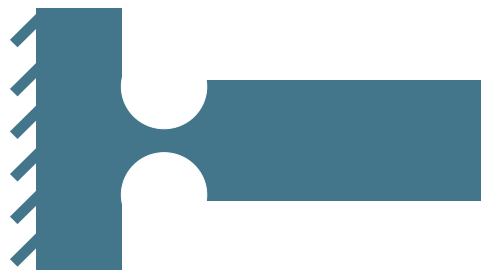
Figure 25 Plan view of cantilever layout with reduced w for breaking stress measurements
