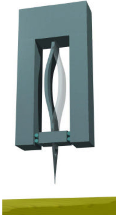
Figure 7-1. Schematic illustration of resonant beam AFM probe with stationary tip.
