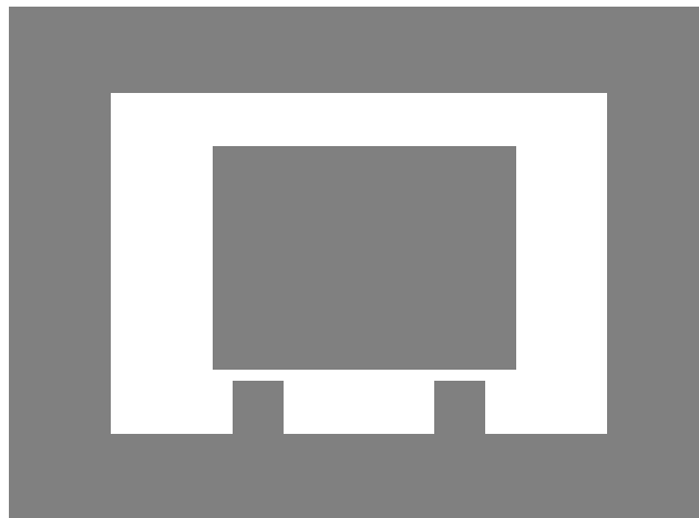
Figure 4-6. Backside release mask for DRIE release. The space between the central chip and the bottom tabs etches more slowly than the rest, so the completed chip is supported by two tabs which are pre-scored to break off cleanly.
