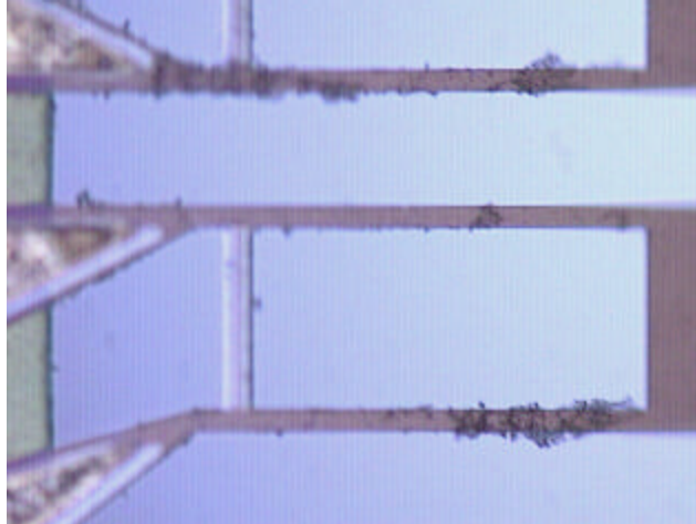
Figure 4-7. Polyimide residue on FABS cantilevers after O 2 plasma release.
